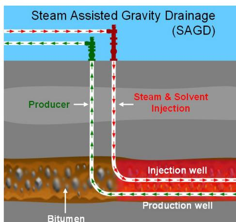
In typical SAGD oil production, water is heated to create steam that mixes with the bitumen and improves its viscosity so it can be pumped to the surface. When solvent is added, the SOR is significantly decreased.
